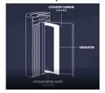
Anode (negative electrode); Cathode (positive electrode); Separator (divides anode and cathode but allows ions to move from side to side)
